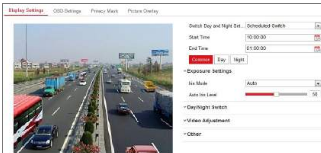
Figure 9-5 Day/Night Scheduled-Switch Configuration Interface
